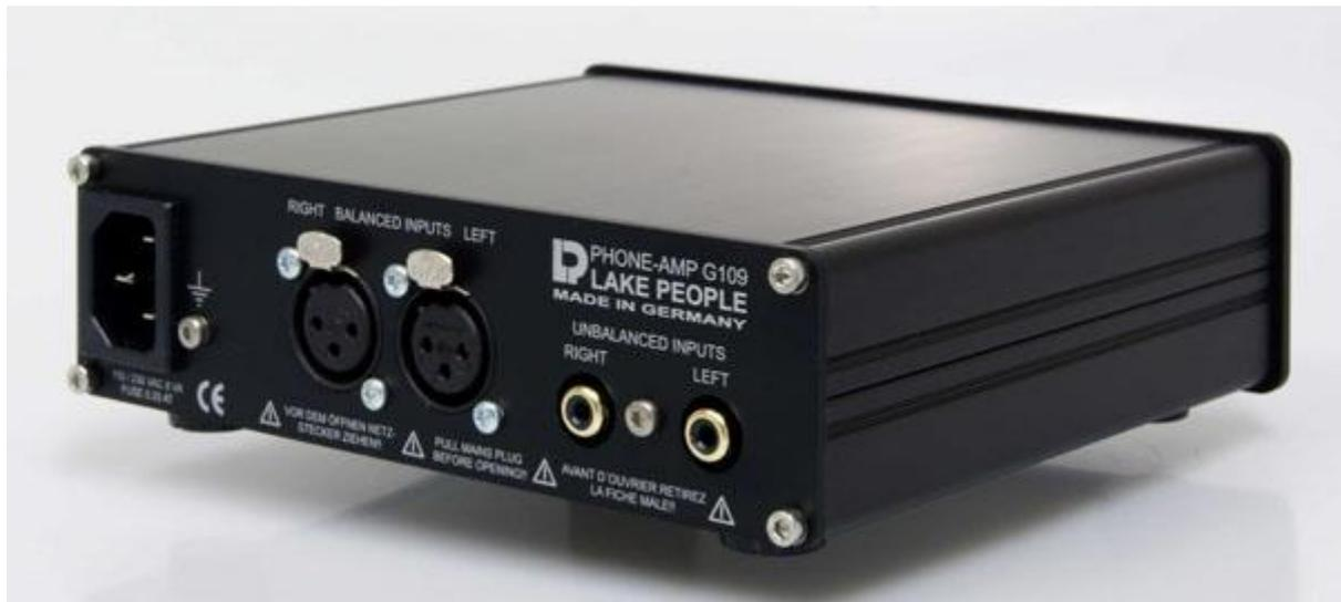
The [Lake People G109](#) is a bit wider than the G103, measuring about 6.5 inches wide, 2 inches tall, and 6 inches deep. The front and rear panels are similar with the exception of inputs, where the G109P keeps both RCA and XLR. The RCA inputs have priority so unfortunately this is still a one-input-at-a-time device.
