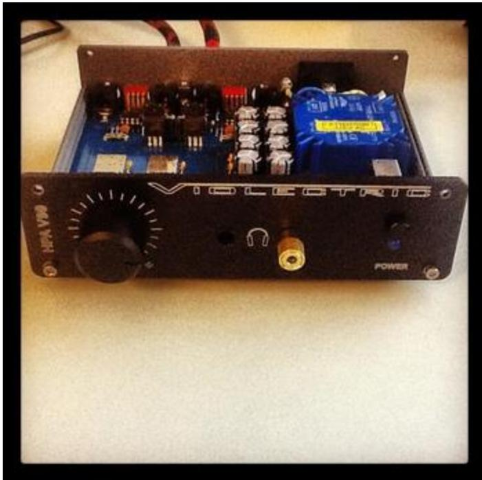
The V90 is the entry level Vioelectric amp and as such is not adorned with the same jewelry as his older siblings. Where the V100, V181 and V200 showcase the brands iconic gold chassis feet, the V90 makes do with simple smallish but chunky black rubber feet. Where the V100, V181 and V200 have 8mm thick aluminum face plates with beveled edges and beveled insets at the headphone jacks and power buttons.... The V90 has a simple flat face plate with headphone jacks and power button surface mounted.
